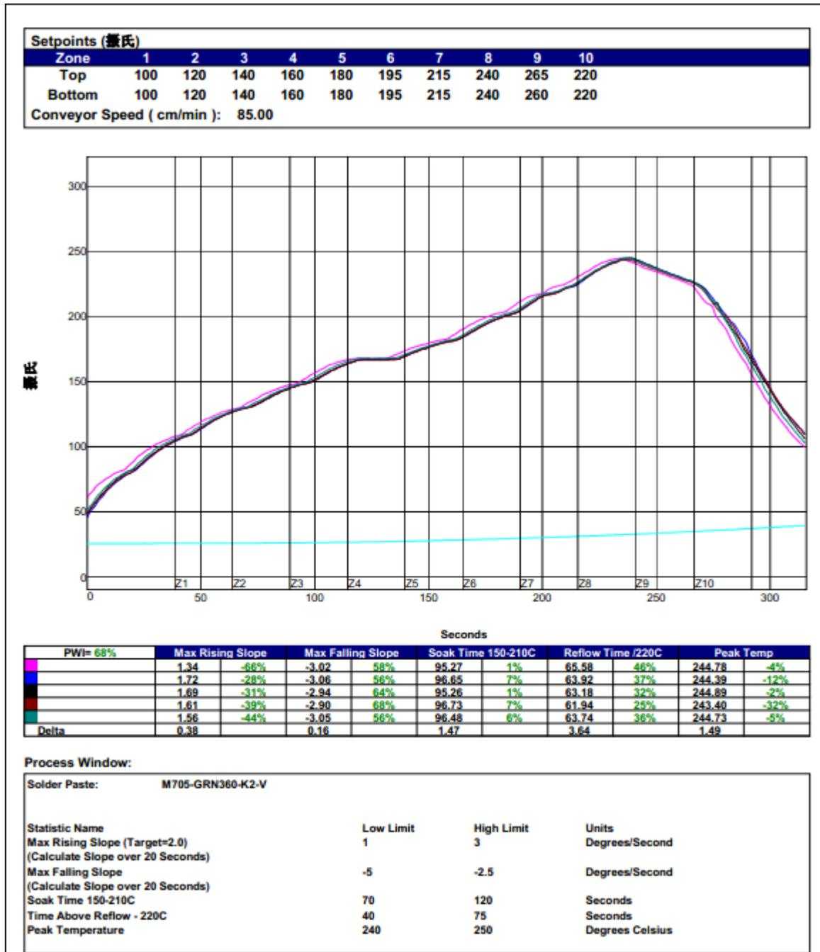
Figure 11: The Ramp-Soak-Spike reflow profile of SIM28
