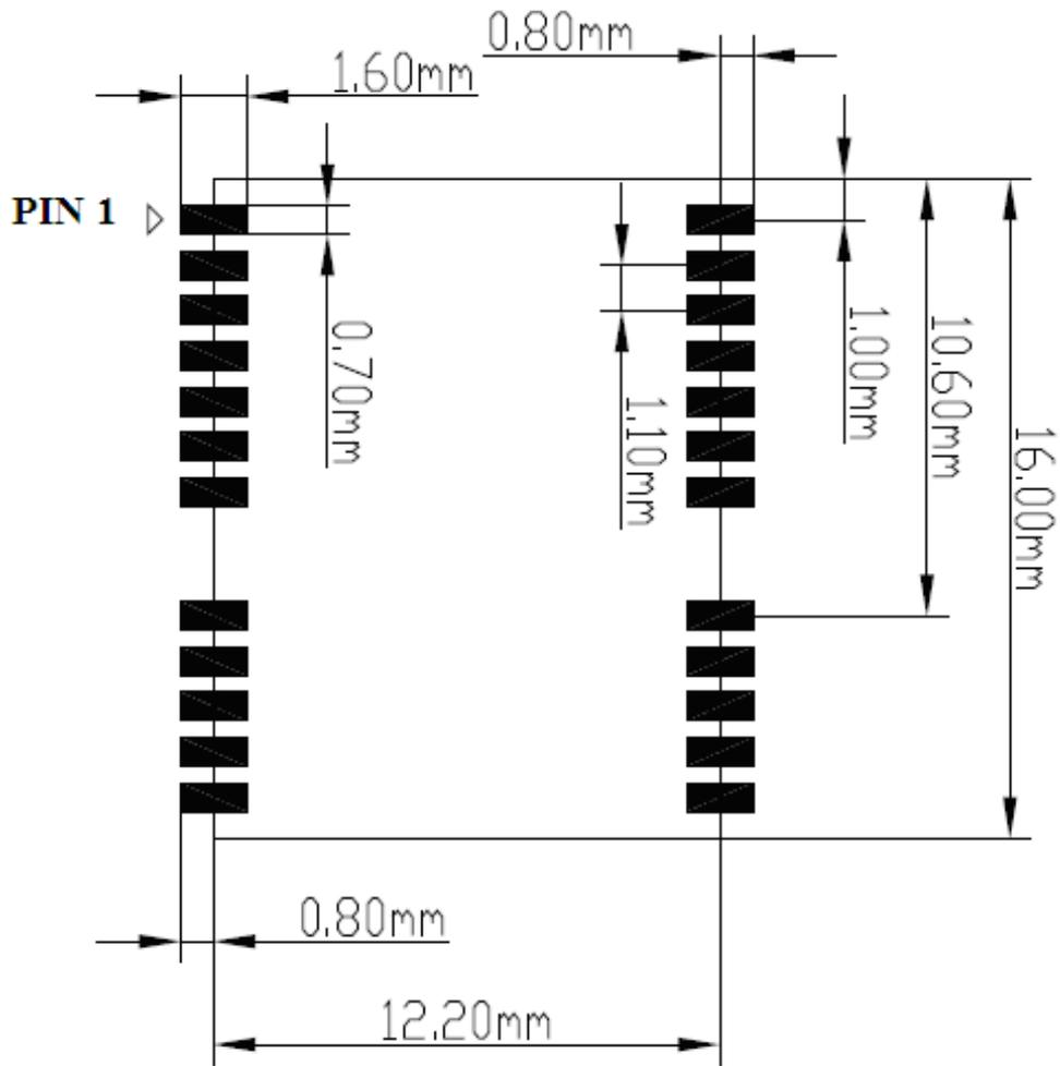
Figure 4: Recommended PCB decal (top view) (Unit: mm)
