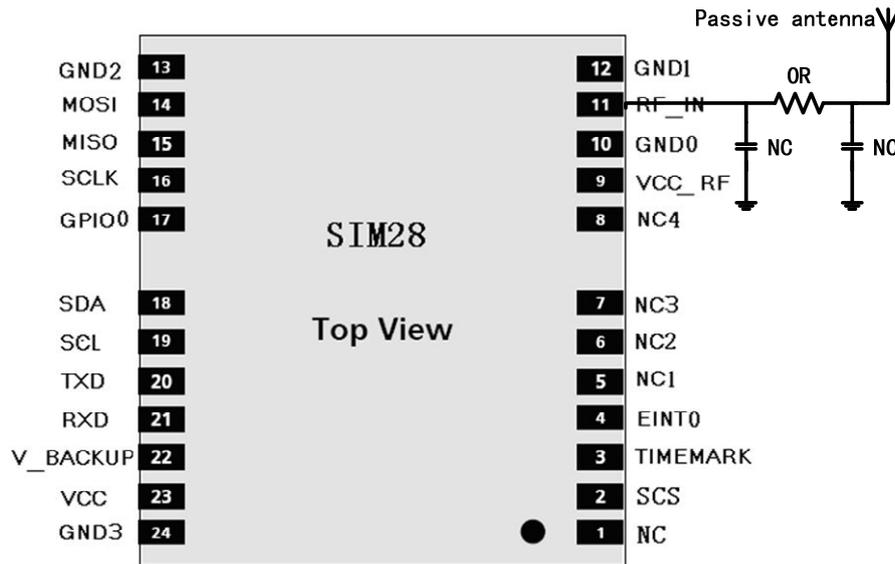
Figure 6: SIM28 passive antenna design
