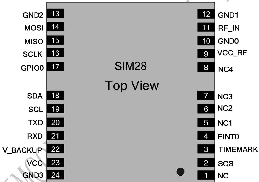
Figure 2: SIM28 pin out diagram (Top view)
