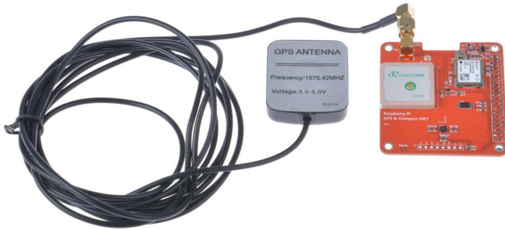
All Ultimate GPS modules have a built in patch antenna - this antenna provides -162 dBm(NEO-6M) or -167 dBm(NEO-M8n)sensitivity and is perfect for many projects. However, if you want to place your project in a box, it might not be possible to have the antenna pointing up, or it might be in a metal shield, or you may need more sensitivity. In these cases, you may want to use an external active antenna.
