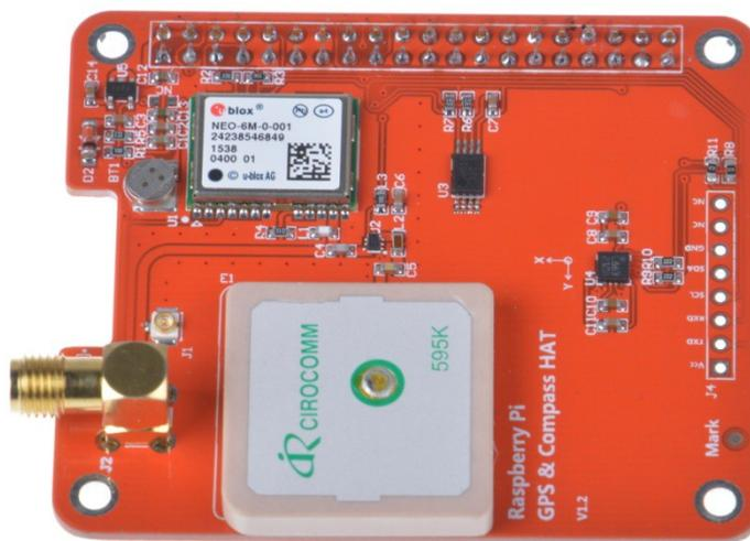
This is an GPS expansion board designed specifically for the both the version 1 and version 2 Raspberry Pi+ Models (This board is NOT compatible with the original Raspberry Pi A and B boards). This board is designed for applications that use a GPS connected via the
